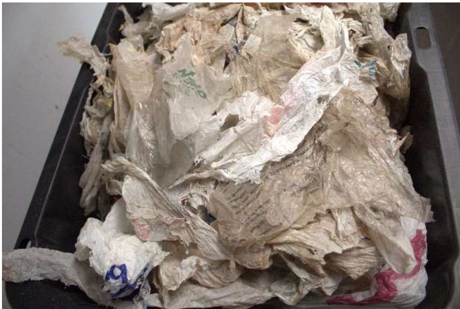
Figure 40: Film extracted from paper using an aspirator and two-inch shaker screen adjusted per the downstream optical.
