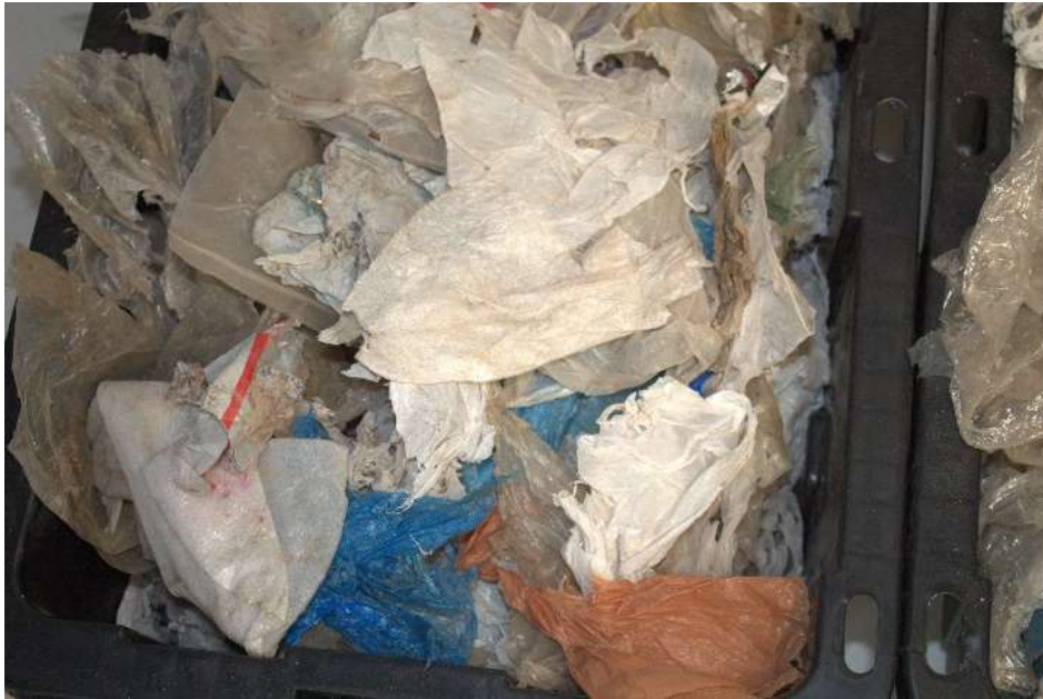
Figure 41: Film ejected via an optical sorter after presentation from the shaker screen and aspirator 24
