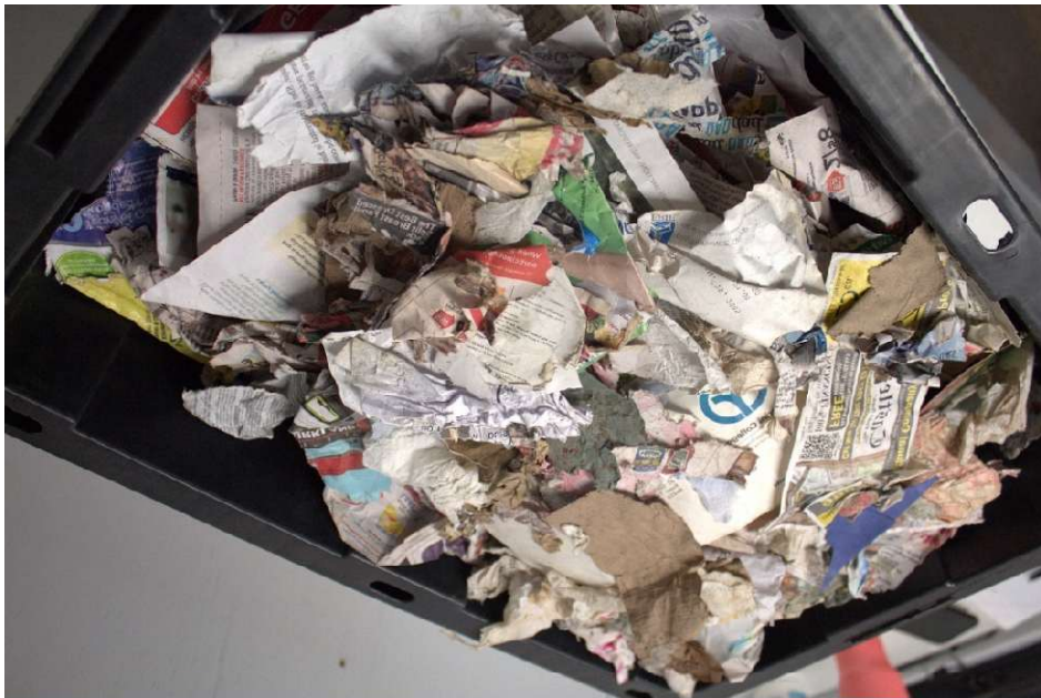
Figure 45. Paper removed via optical sorting from the Hefty ReNew™ Bags.
