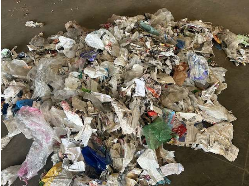
Figure 40: Film extracted from paper using an aspirator and two-inch shaker screen adjusted per the downstream optical.
