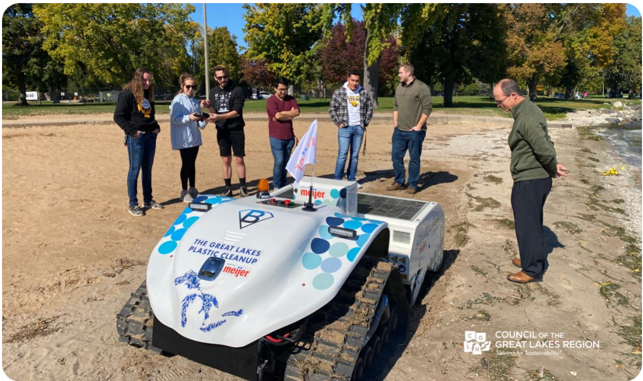
Photo: A BeBot in action cleaning up plastic debris and waste from a Great Lakes shoreline.
